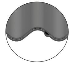
Optional anti-Siphon channel prevents water from penetrating the overlap.
