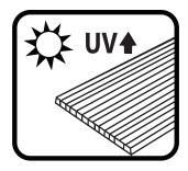
**Note:** The masking film on the polycarbonate sheet indicates which side of the sheet is UV protected. **The blue film indicates the exterior side which is UV protected.**
