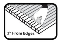
**Note:** If the masking is stuck to the sheet, rub with a soft cloth wetted with Fels-Naptha or isopropyl alcohol. Pull off the film and follow immediately with a mild soap cleaning and a thorough water rinse. Do not use sharp objects or other chemicals to remove masking.
